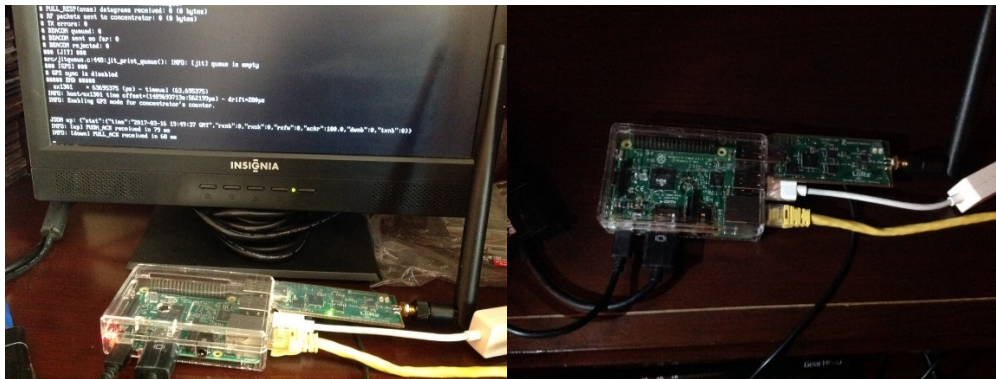
Figure 6- LoRaWAN Test Device Prototype
